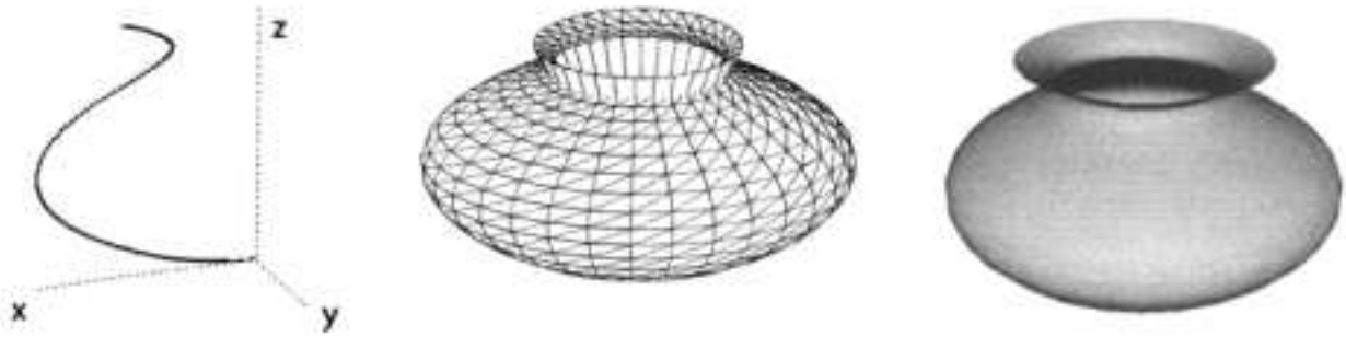
Figure 3.4: Rotational Sweep: a profile curve, the surface of revolution, and the shaded image
